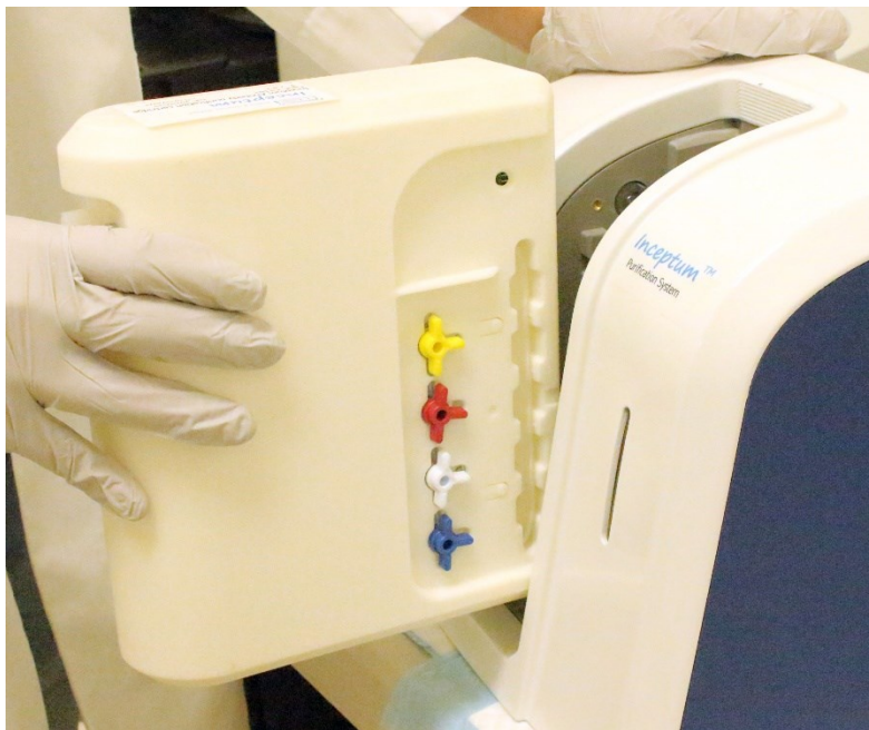
Figure 9. Insert cartridge into the instrument slot as shown above. The cartridge should slide into the slot without excessive force. If there is difficulty inserting the cartridge, check the correct orientation of the valves (see previous step) or turn instrument off, then on to realign valves.
